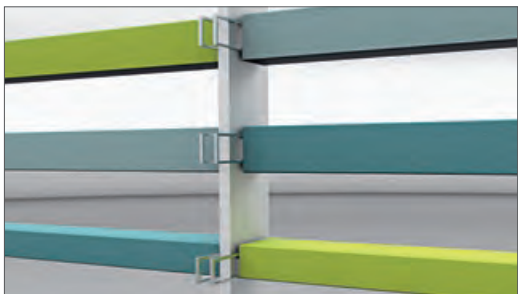
Slide securing clip on the base plate
